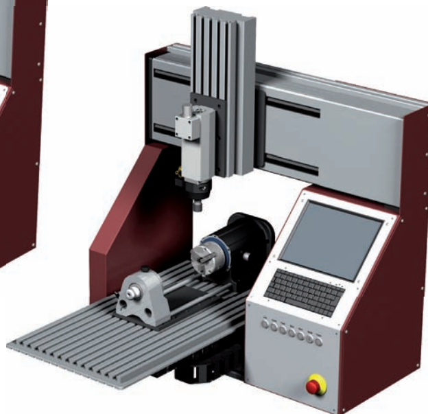
Figure: MiniMod V 60 with milling spindle and rotary axis RDH-S with tailstock
